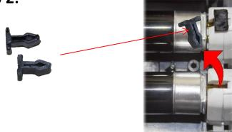
Turn the unit upside down. Remove the clips by pulling them out from either side of the globe.
